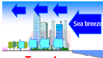
Type-1 Ventilation path - along ground level
