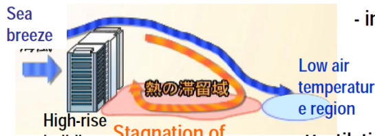
Type-3 Ventilation path - induced by high-rise buildings
